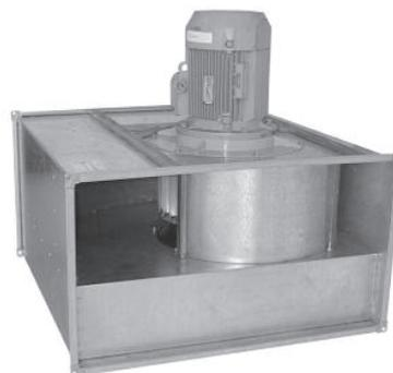
ВРПВ-Н КХ (VRPV-N KH) fans are designed for operation in the kitchen exhaust systems and local exhausts of other manufactures for the purpose of handling air at the temperature of up to +200 °C and increased humidity.
