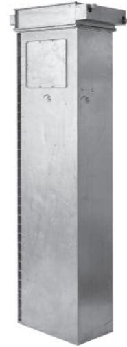
ZVV air curtains are designed for gateways protection against sweep of warm or cold outside air through opening with area of 4 m<sup>2</sup> and more by means of forming of an air jet in the gate opening plane. Air jet moving from the curtain slot mixes with outside air on one side and with inside air on the other side gaining definite average temperature.
