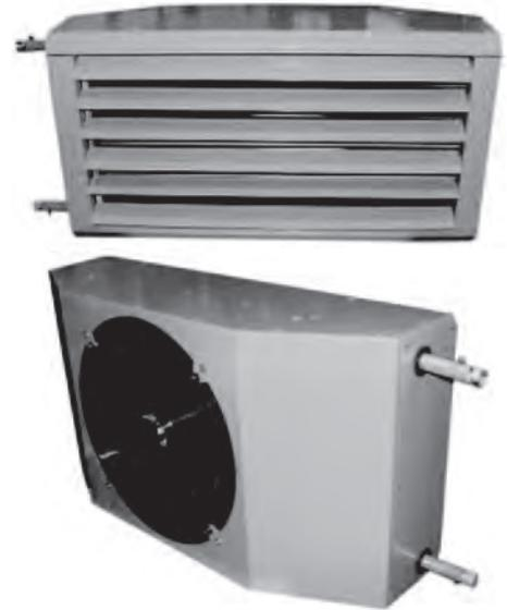
Attached heating and ventilation units HOBA (NOVA) are designed for air heating using hot water circulating through aluminum-copper set heat exchanger (heating), and homogeneously distributing of air in a room using fan and guide vanes. Components are designed for operation in inside air. Heat-carrying agent shall not contain substances chemically active towards copper and steel.
